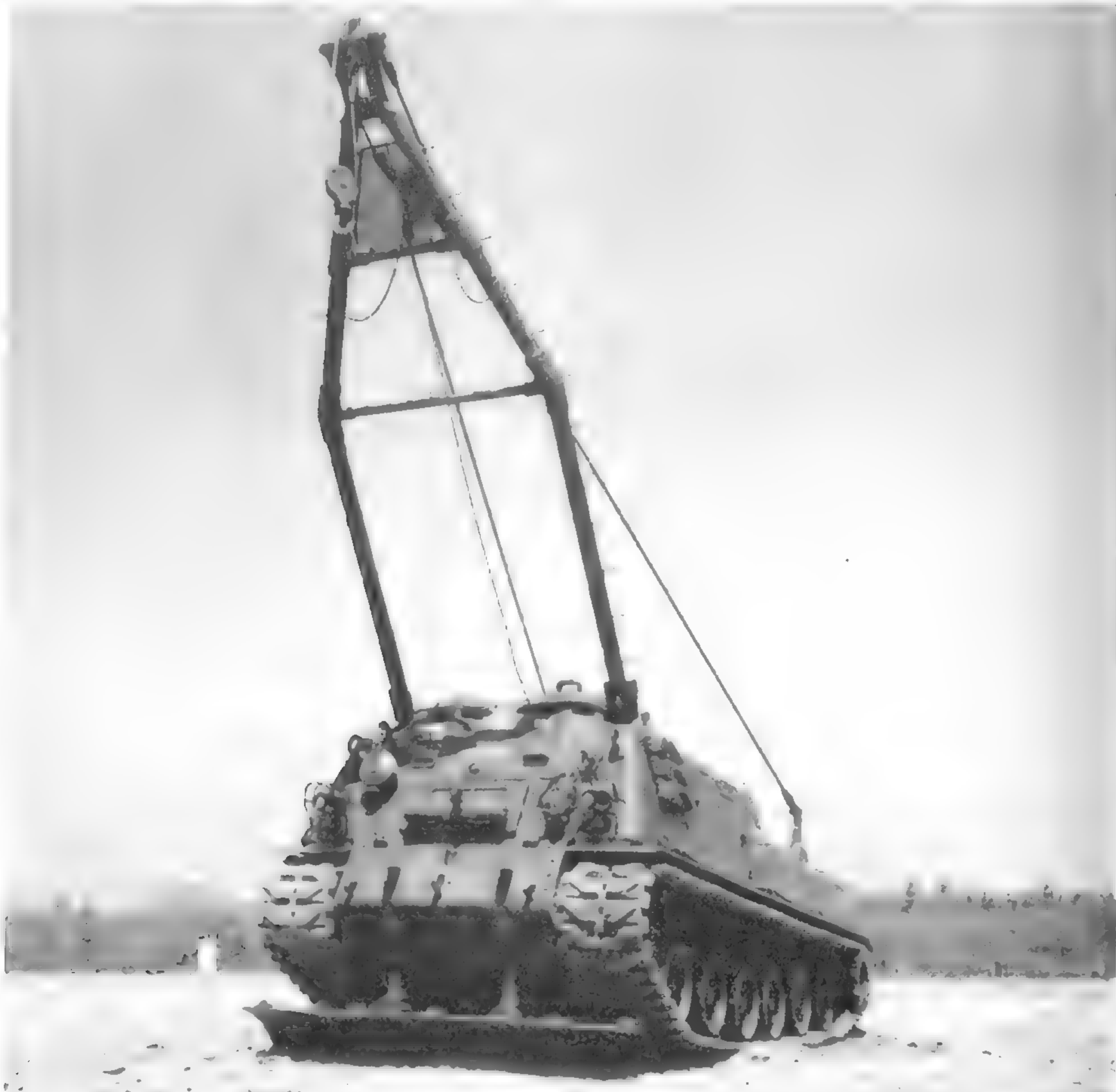
The A-frame of the M88 has been raised in this view, and the front anchor spade lowered. While sometimes used for bulldozing, it is for use such as this that the spade was installed on the vehicle. During winching operations it could be partially lowered to serve as a ground anchor, or during lifting operations it was lowered completely so the lifted load was transmitted directly through it to earth. This prevented overloading the M88s torsion-bar suspension system. (Photo courtesy of the Patton Museum)
